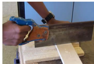
Using a bench hook for sawing.
